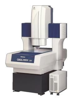
Westech has added two **Mitutoyo QV404 Automated Vision Inspection Systems** to its onsite inspection facilities in the UK and US which extend its capability to perform the mensuration of all impaction devices including the ACI, the NGI and the Westech W7 using the parameters set out by the instrument manufacturers or the relevant international Pharmacopeia.
